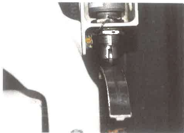
Figure 14-119. Main landing gear with Weight On Wheels (WOW) sensors.
