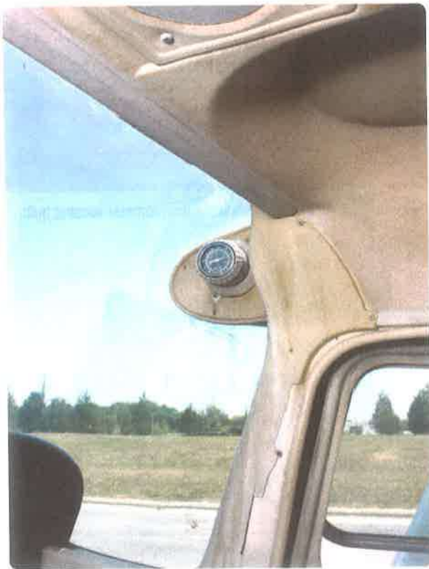
Figure 7-66. A bimetallic outside air temperature gauge.
