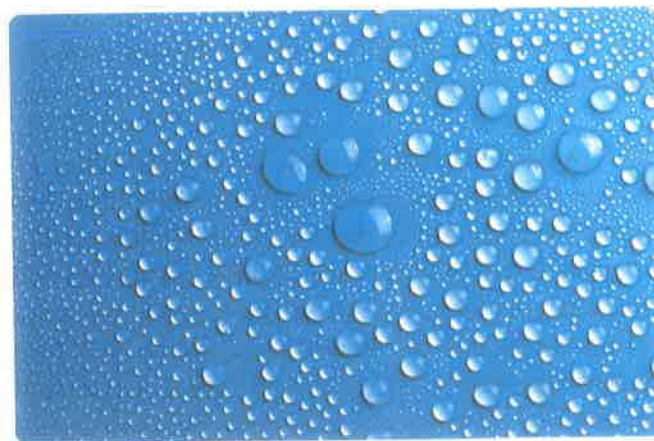
Figure 13-18. Rain repellent causes water to 'bead-up'.
