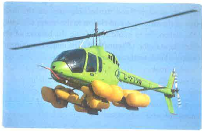
Figure 9-18. Emergency floats deployed on a Bell 505.
