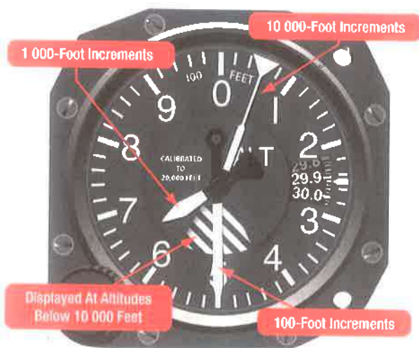
Figure 7-16. A sensitive altimeter with three pointers and a crosshatched area.
