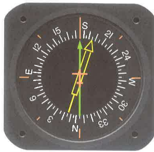
Figure 7-104. A radio magnetic indicator (RMI).
