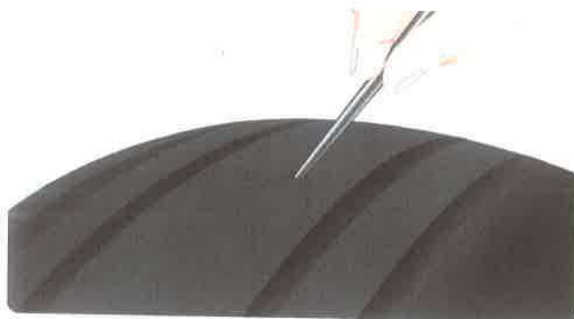
Figure 14-71. Removal of FOD.
