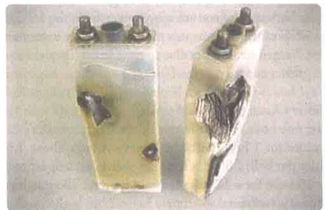
Figure 8-5. Thermal runaway damage.
