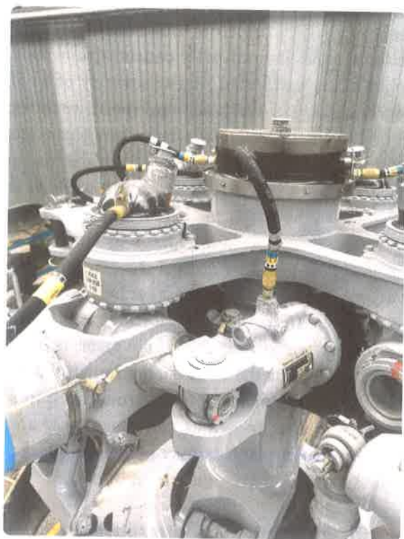
Figure 2-35. Drag hydraulic damper on SA330 puma.
