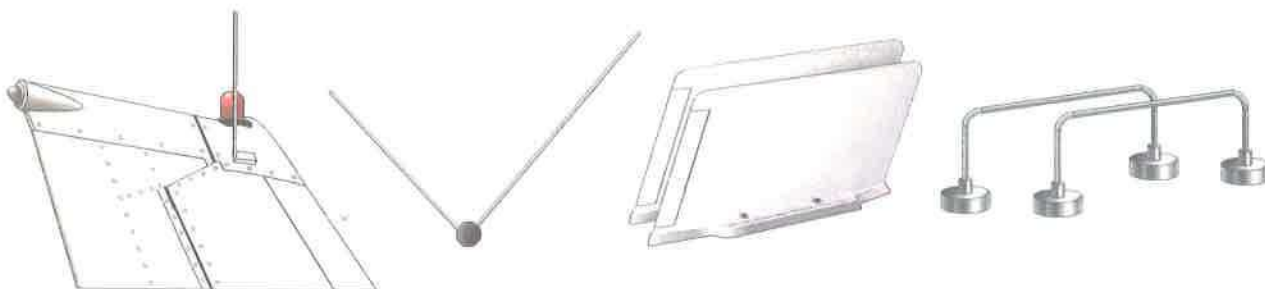
Figure 7-93. V-shaped, horizontally polarized, bi-pole antennas.
