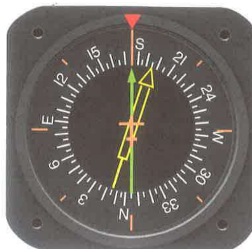
Figure 7-48. A radio magnetic indicator (RMI).
