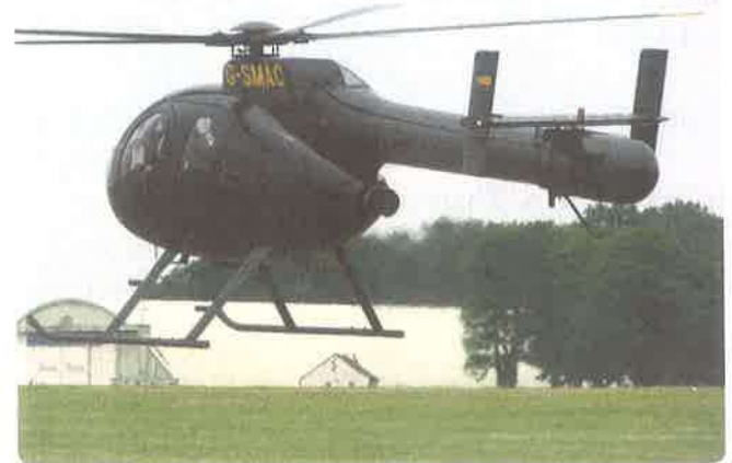
Figure 2-29. MD-520 helicopter with no tail rotor.
