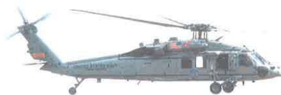
Figure 1-16. Tilt of main rotor during forward flight (Sikorsky H-60).
