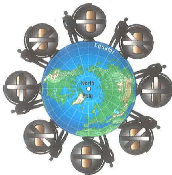
Figure 7-27. Once spinning, a free gyro rotor stays oriented in the same position.
