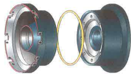
Figure 14-52. Two-piece split-wheel aircraft wheels.
