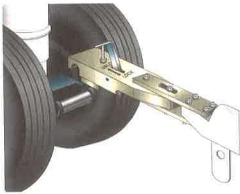
Figure 14-26. A towing lug on a landing gear.
