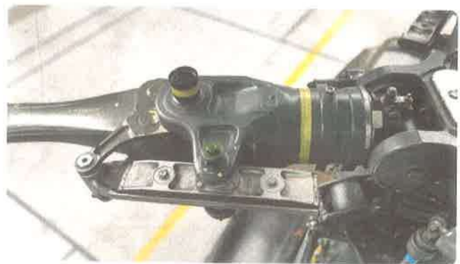
Figure 2-40. Elastomeric damper on SA341 Gazelle.
