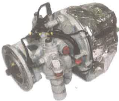
Figure 12-4. Hydraulic power pack.
