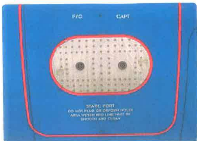
Figure 7-13. Heated primary and alternate static vents.
