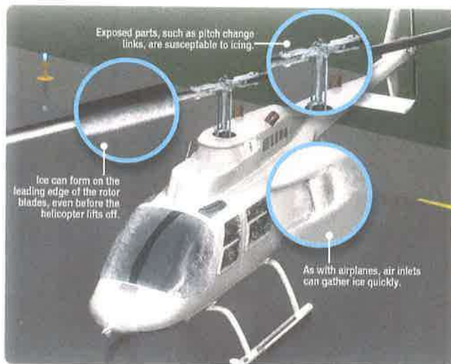
Figure 13-1. Ice formation can effect various parts of a helicopter structure.
