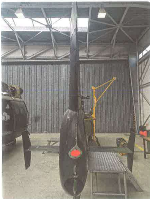
Figure 2-28. Fenestron dissymmetric vertical fin.
