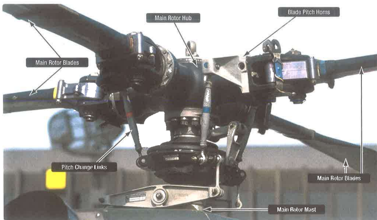
Figure 2-38. Four-blade hingeless (rigid) main rotor.
