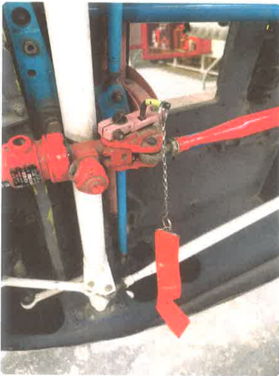
Figure 2-78. Relay locked by a pin.
