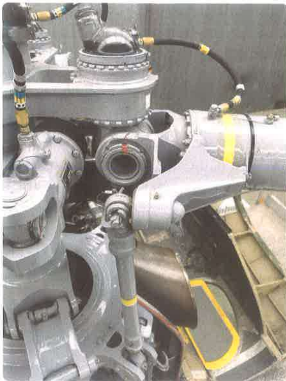
Figure 2-33. Fully Articulated Main Rotor System.
