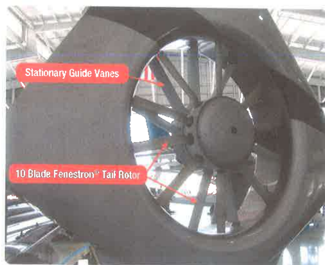
Figure 2-51. Fenestron tail rotor for an EC-135 helicopter.
