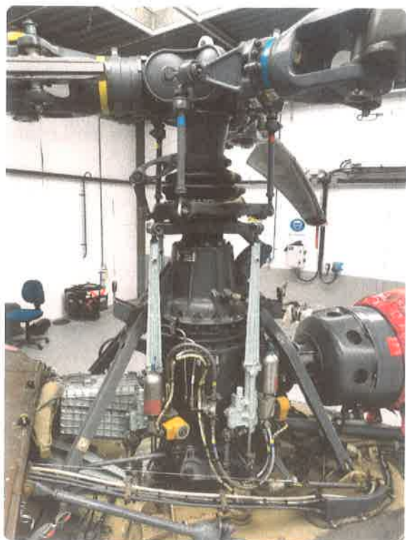
Figure 2-82. Pitch change rod and actuator control rod of the servocontrols.
