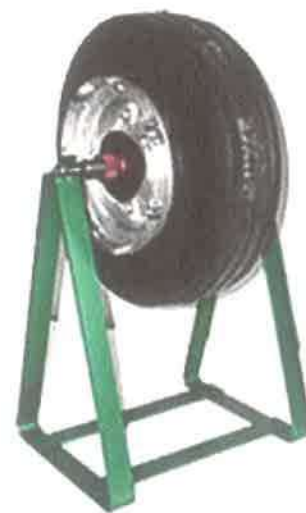
Figure 14-85. A typical aircraft tire and wheel static balancing stand.
