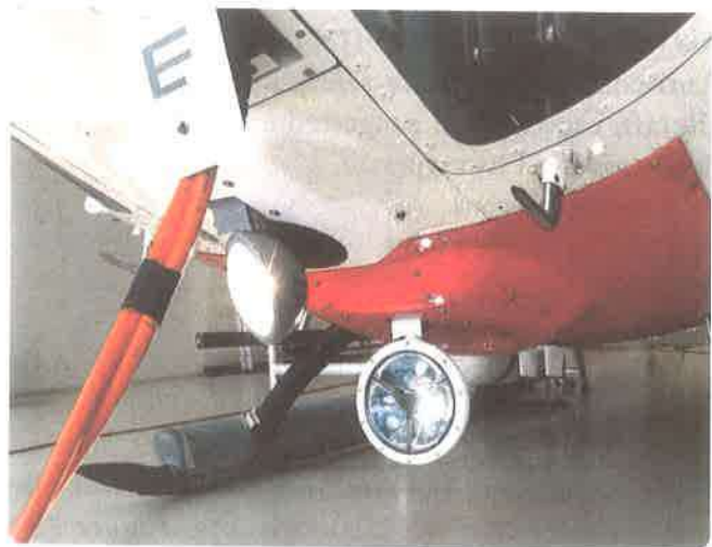
Figure 15-14. A combination landing and rotatable search light on an airbus BK 117.
