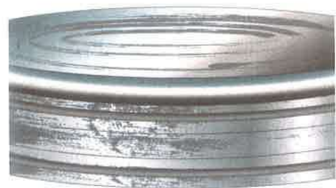
Figure 14-59. Loose bearing cup damage.
