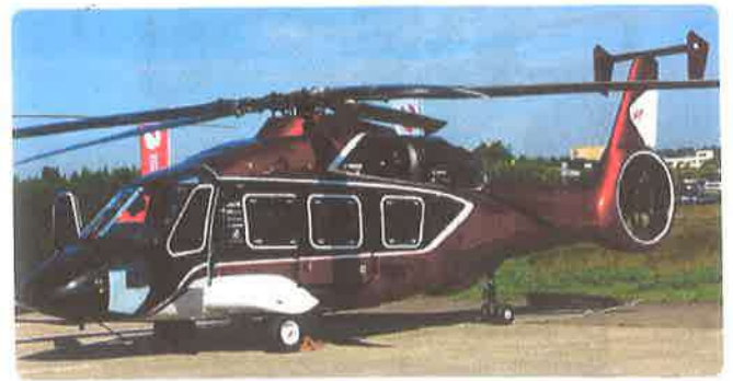
Figure 14-4. A tail-wheel type landing gear.
