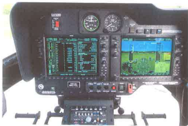
Figure 7-5. A secondary airspeed and altimeter provides redundancy for the digital displays.
