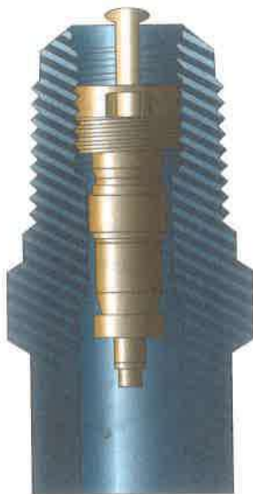
Figure 6-15. R12 refrigerant valve.
