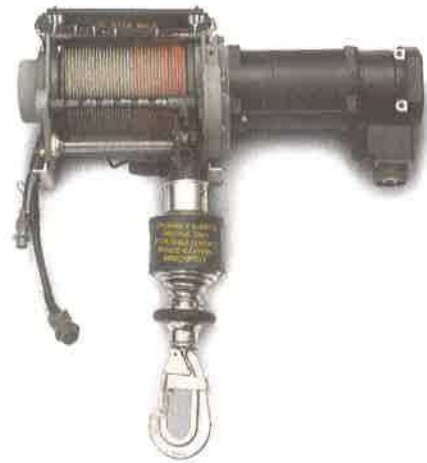
Figure 9-12. A hoist mechanism rated for 200 Kg (450 pounds).
