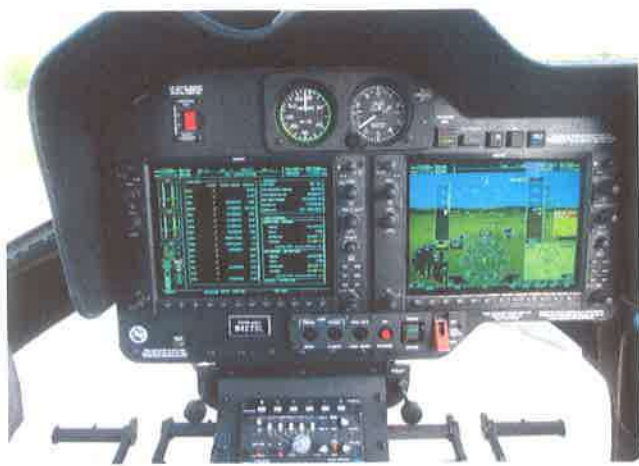
Figure 17-2. IMA display panel on a newer Bell 407.
