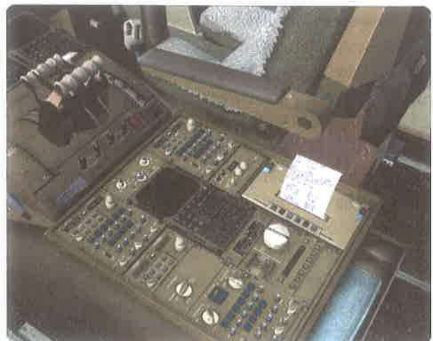
Figure 18-8. An ACARS compatible flight deck thermal printer.
