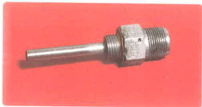
Figure 7-67. An electric resistance thermometer sensing bulb.
