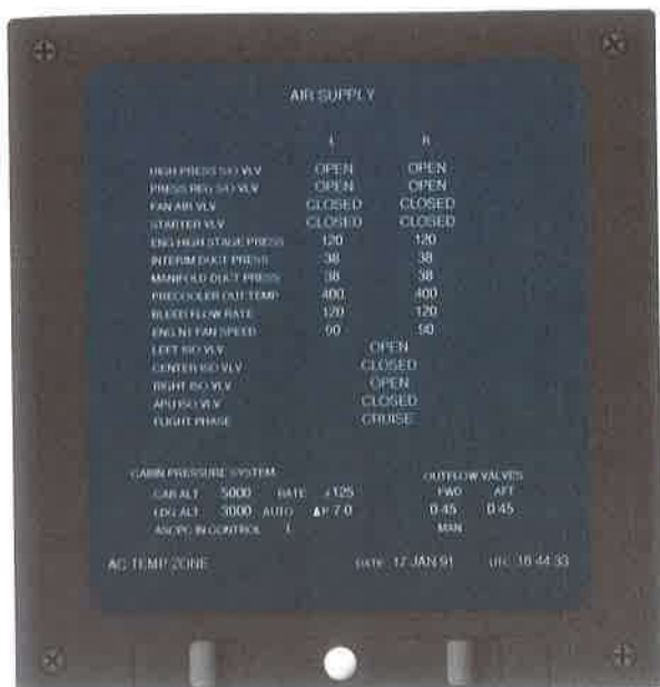
Pneumatic Air Supply Display
