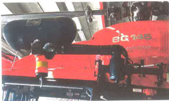
Figure 9-11. An electric hoist capable of lifting people and other lighter objects.
