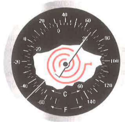
Bimetallic coil of bonded metals with dissimilar coefficients of expansion.
