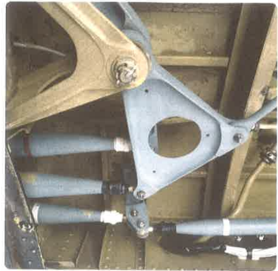
Figure 2-81. Fixed and semi-adjustable rods.
