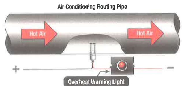
Figure 6-36. Over heat detector.
