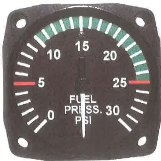
Figure 7-82. A typical analog fuel pressure gauge.
