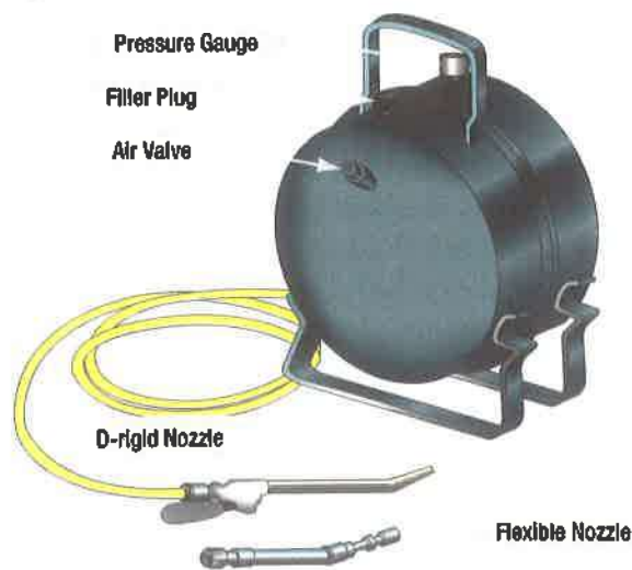
Figure 14-107. A typical brake bleeder pot or tank.
