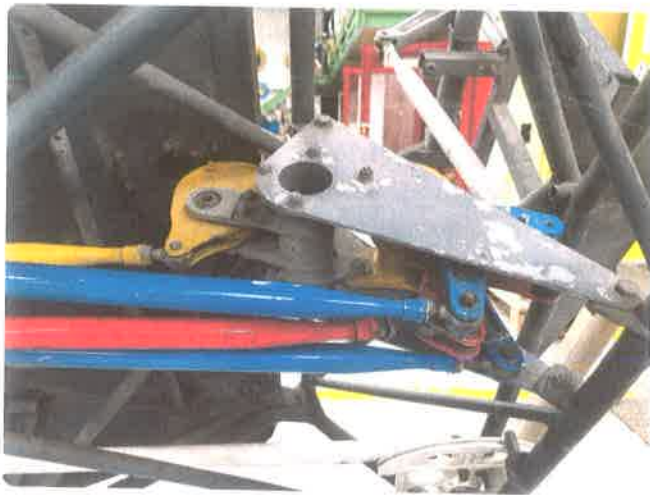
Figure 2-67. Rods and bellcranks on the mixer unit.
