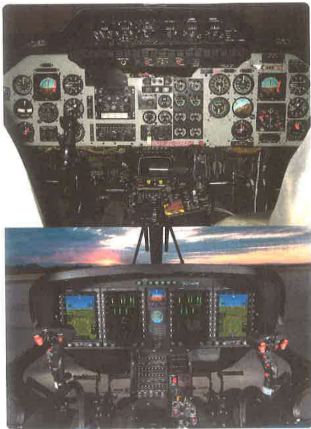
Figure 7-2. A conventional panel of a Bell 222 and modern glass panel of a Leonardo TH-119.
