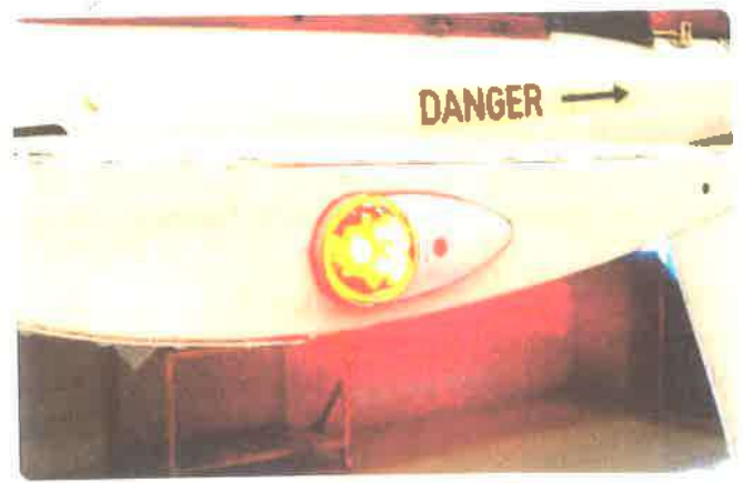
Figure 15-9. A typical anti-collision light installation in a vertical stabilizer.
