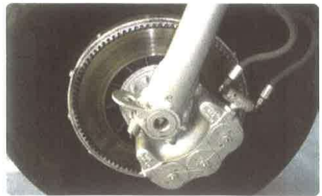
Figure 14-89. A single disc brake; floating-disc, fixed caliper.
