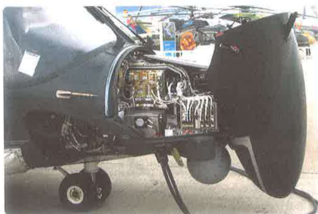
Figure 7-90. Communications and other devices in an avionics bay.
