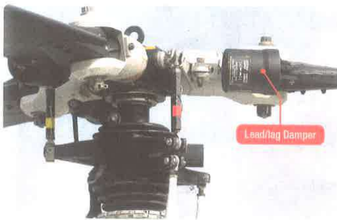
Figure 2-39. Fully articulated main rotor with lead-lag damper.
