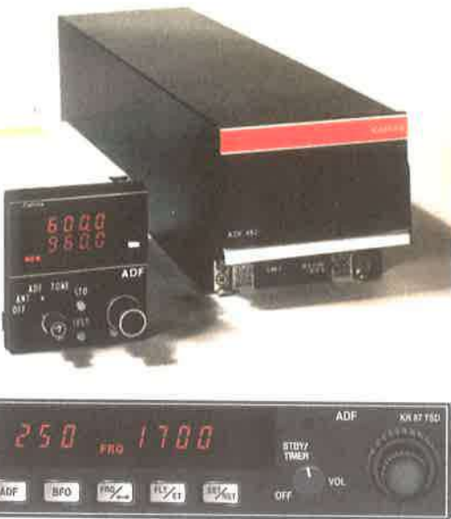
Figure 7-103. A cockpit mountable ADF receiver.
