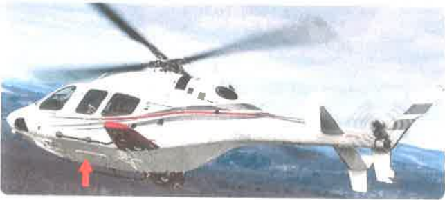
Figure 14-12. Fitting panels on retractable landing gears.
