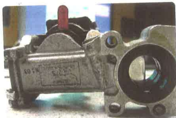
Figure 11-13. This motor-operated gate valve has a red position indicating lever.
