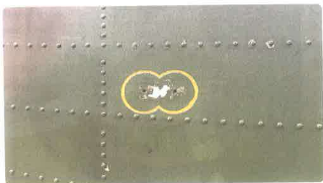
Figure 7-20. The location of the static vent.
