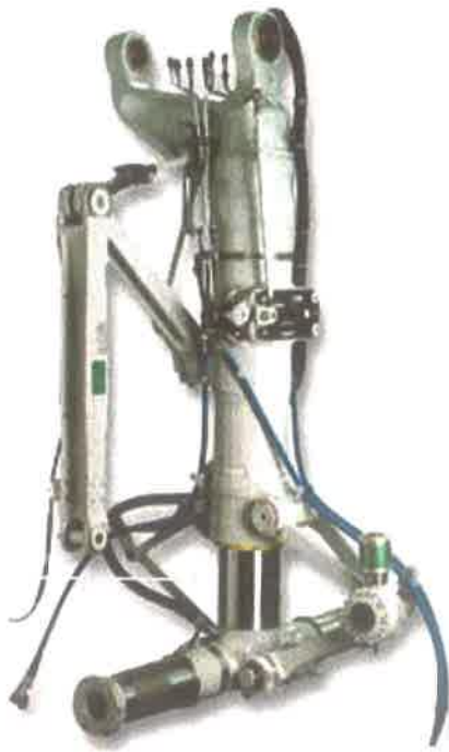
Figure 14-23. Axles machined out of the same material.
