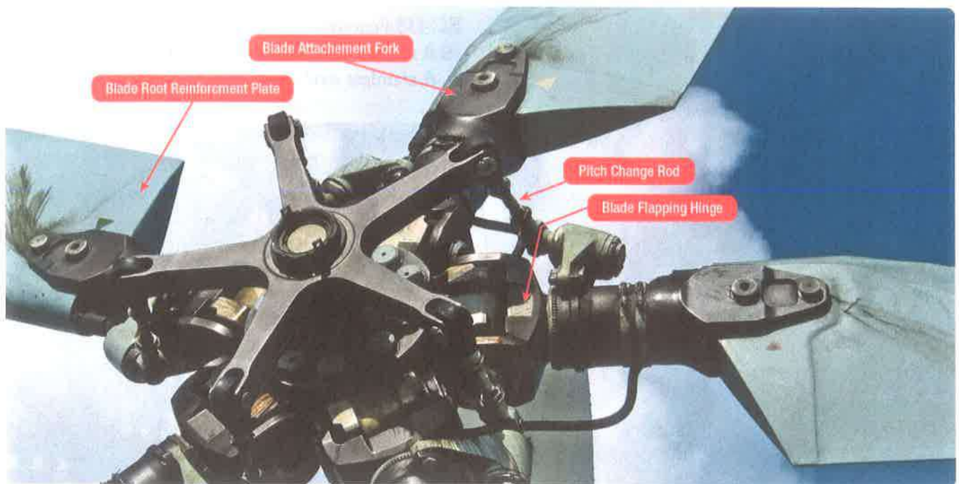
Figure 2-49. Tail rotor assembly on a MIL MI-26 helicopter.
