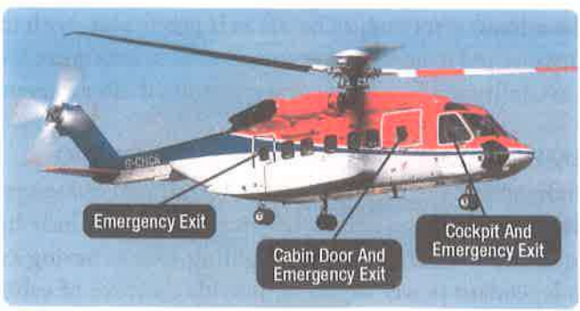
Figure 9-6. Emergency exit locations showing their banded external markings.
