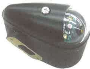
Figure 15-8. A forward position LED position light from Devore Aviation.
