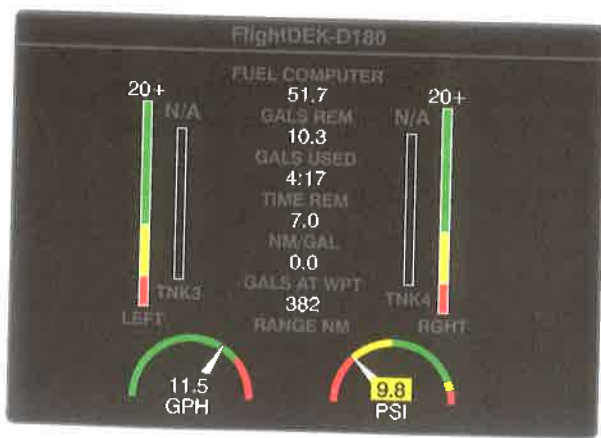
Figure 11-46. An electronic display of fuel parameters.
