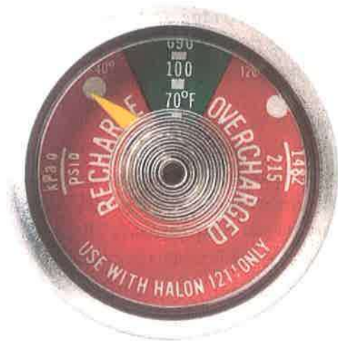
Figure 10-19. A gauge showing an extinguisher is need of service.
