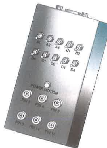
Figure 7-124. A handheld transponder test unit.
