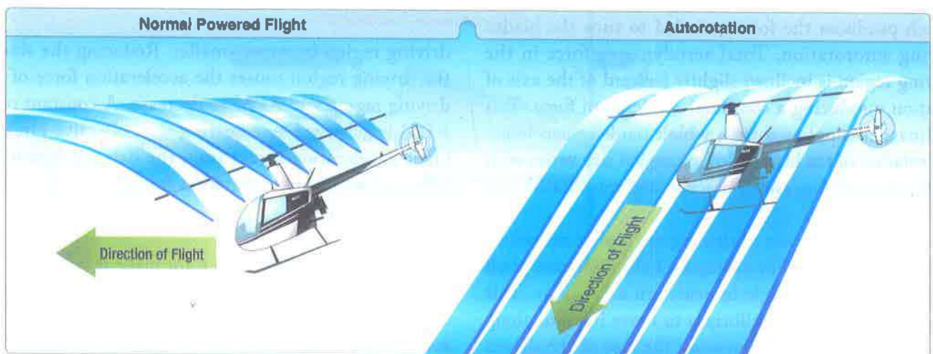
Figure 1-25. Main rotor airflow during normal flight and autorotation.
