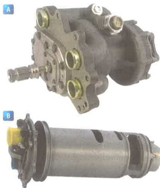
Figure 11-8. (A) An engine driven fuel pump from Eaton Aerospace. (B) An electric fuel boost pump from Crane Aerospace.
