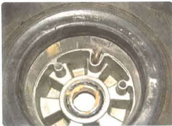
Figure 14-84. Mounting a tube type tire on an outboard wheel half.
