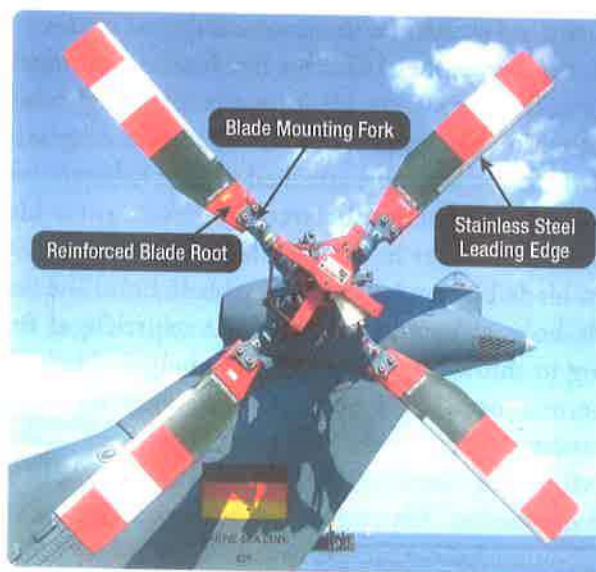
Figure 2-47. Tail rotor blade attachment on a Westland Sea Lynx helicopter.
