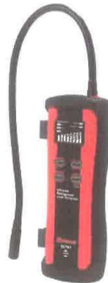
Figure 6-23. Infrared leak detector.
