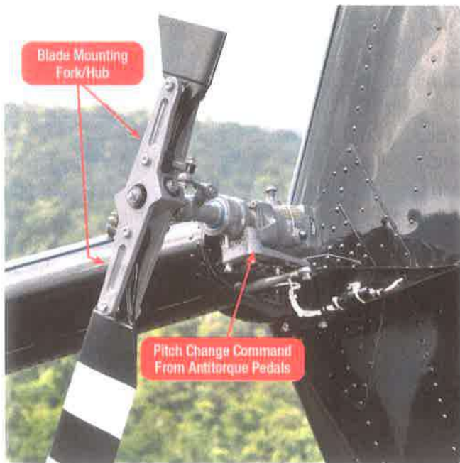
Figure 2-48. Tail rotor blade attachment on a Robinson R-44 helicopter.
