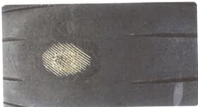
Figure 14-73. Tire damage caused by landing with the brake on.
