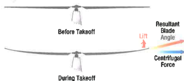
Figure 1-23. Coning of main rotor during takeoff.
