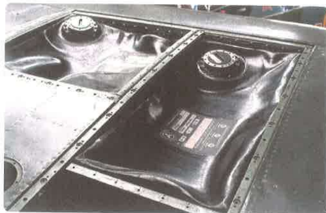
Figure 11-6. Bladder fuel tanks, each with its own filler, placed in compartments within an aircraft structure.
