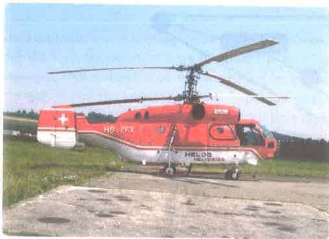
Figure 2-25. Helicopter with coaxial counter-rotating main rotors.
