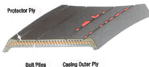
Figure 14-76. Tread chipping and chunking.
