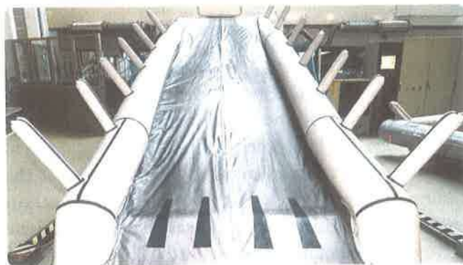
Figure 9-7. A self-deploying emergency exit slide, also suitable as a raft.
