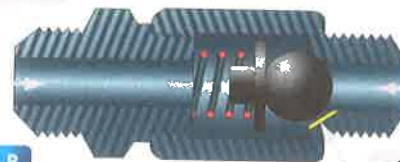
Orifice-Type In-line Check Valve (Ball-Type)
