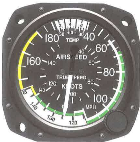
Figure 7-22. An analog true airspeed indicator.
