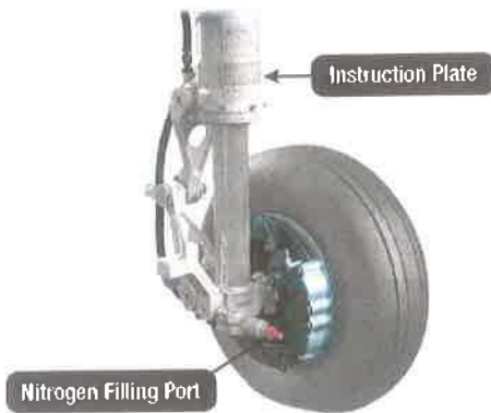
Figure 14-27. Instruction plate and Nitrogen filling port.
