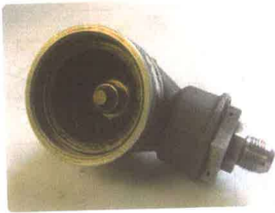
Figure 10-13. Discharge valve (left) and cartridge, or squib (right).
