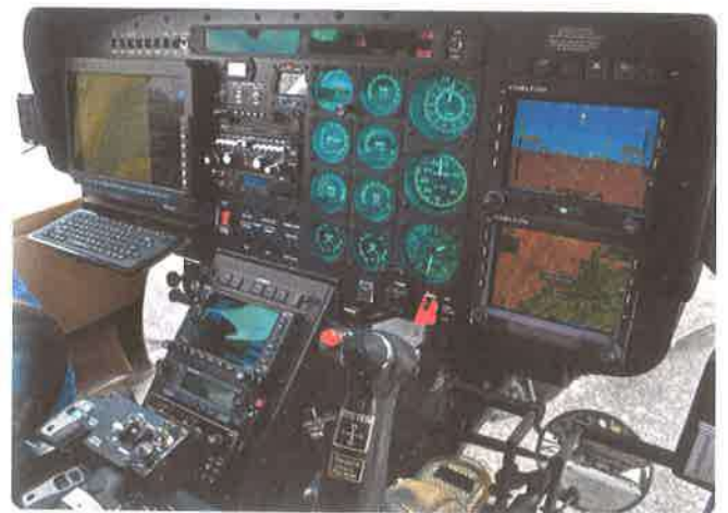
Figure 7-7. Engine and other common instruments placed between pilot and copilot of this Hughes MD-500.
