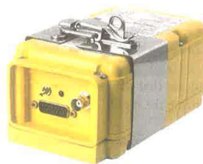
Figure 9-4. An Emergency Locator Transmitter.
