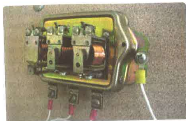
Figure 8-23. The three relays found on this regulator are used to regulate voltage.
